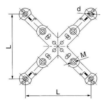
The clamps are aluminum alloy.Daanpeys are clastomer.The other parts are hot-dip galvanized steel.
